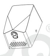
**Installation and setup:** It should be done by a qualified electrician. It has to be minimum 1,1 m between the floor and the hand dryer base. Do not install the hand dryer on a shiny surface. Place template against the wall at desired height and mark location with 4 mounting holes (8 mm - diam.). Before replacing the cover, there is an option to run the dryer heater on 1350 W or heater off 500W. The switch is clearly marked.
